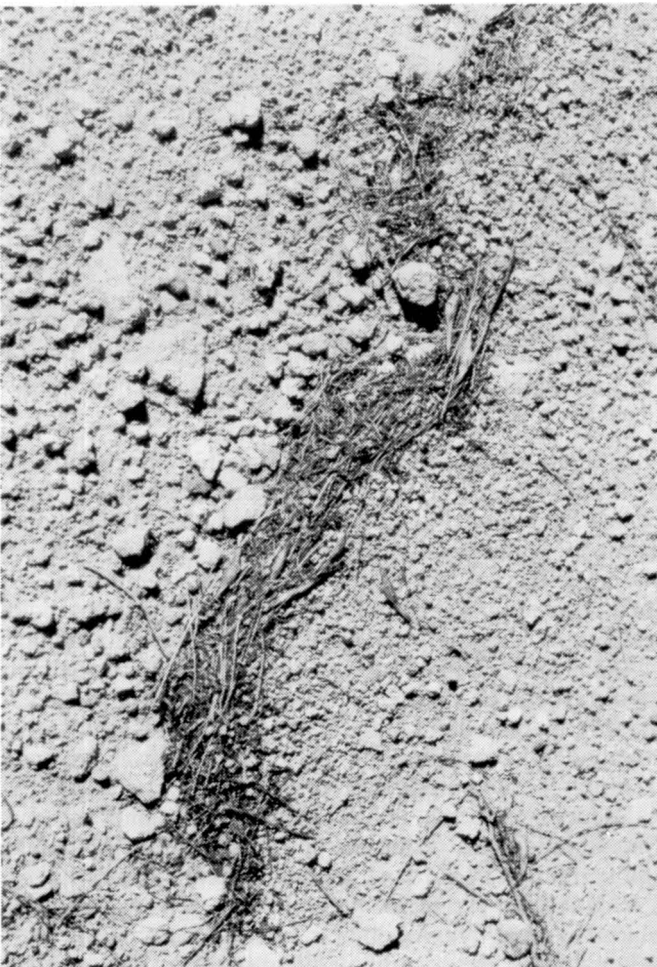
Runoff flow is from right to left. Note smaller-grained sediments trapped behind the organic dike.
